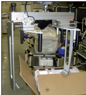
Special tool for lifting printers
