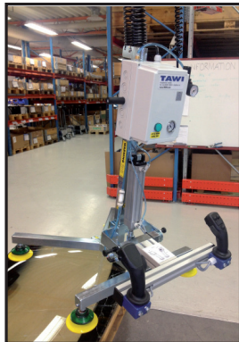
Lifting glass car wind- shields using dual joystick control
