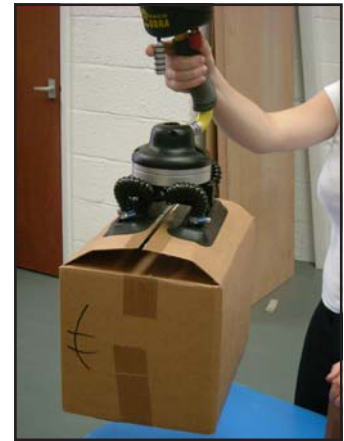
VacuCobra with adapter for VM120 suction foot art nr 30620. A better choice for poorly taped boxes.
